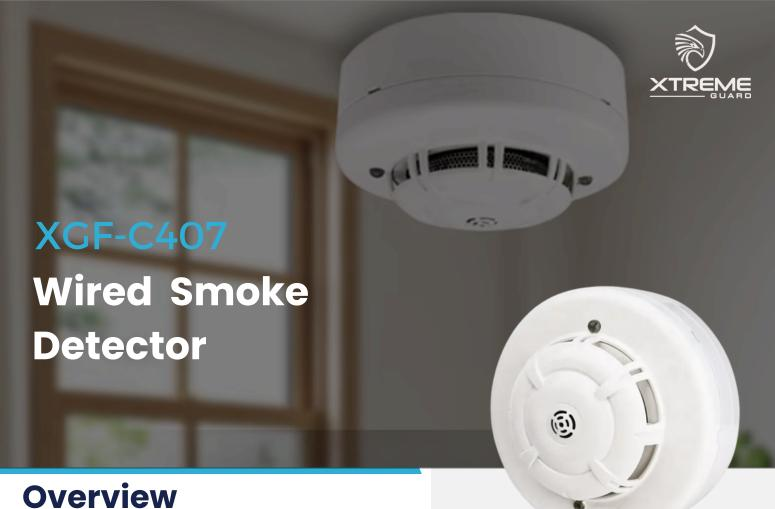
The XGF-C407 is a high-performance wired photoelectric smoke detector, designed for integration into 2-wire or 4wire fire alarm systems. Built for precision, safety, and longterm reliability, the detector offers accurate smoke detection using photoelectric sensing and features a builtin audible alarm of over 80dB at 1 meter, providing both visual and sound alerts for timely evacuation.
